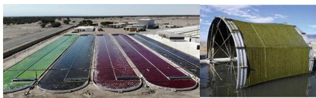
Figure 1 – Astaxanthin production (in red) in open-ponds (Figure on the left). Rotating biofilm-based systems at pilot scale (Figure on the right), (Bernstein et al., 2014)
