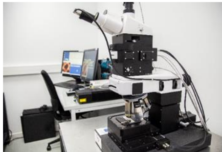
Figure 1. Microscope confocal Raman Alpha 300R+, Witec
