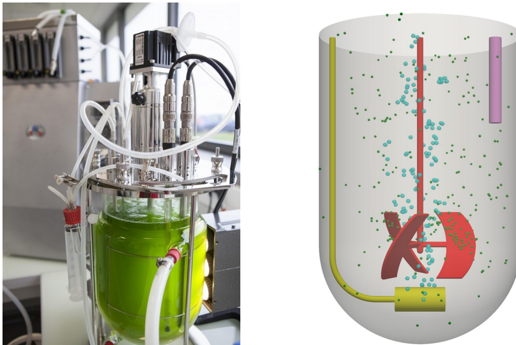
Fig. 2: 5-liter stirred tank photobioreactor (left), numerical simulation (right)
