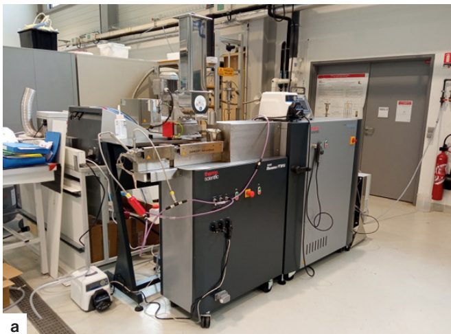
(a) Twin screw extruder enables the elaboration of new biomaterials, the extraction of molecules of interest from biomasses and reactive extrusion to be carried out by adding various reagents and enzymes. It's a versatile tool calibrated for research and scale-up. (b) example of a new biocomposite produced with agro-industrial by-products to substitute traditional plastics.
