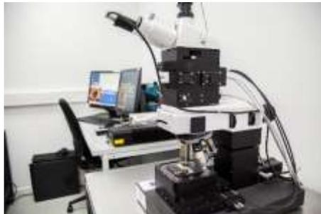
Figure 1. Microscope confocal Raman Alpha 300R+, Witec
