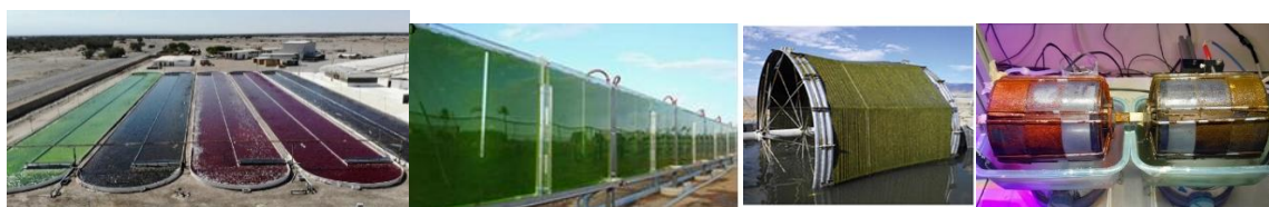
Figure 1 - Astaxanthin production (in red) in open-ponds (Figure on the left). Closed photobioreactor (Figure on the middle). Rotating biofilm-based systems at pilot and lab-scales (Figures on the right), (Bernstein et al., 2014, Morgado et al., 2023)
